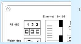
The pin (3) is Not connected
