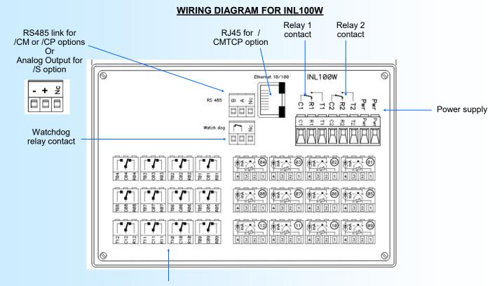
Channel alarm relay contact.
